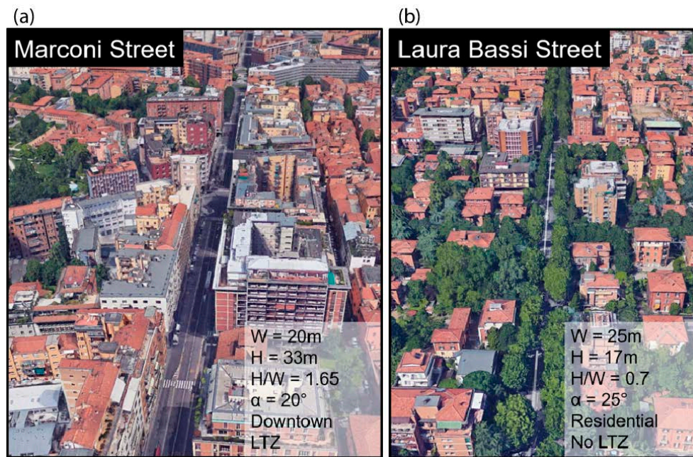
Figure 2. Street canyons views and details ( W = mean street width, H = mean street height, \alpha = orientation angle of the street canyon with respect to the meteorological north, LTZ = Limited Traffic Zone) of the two street canyons in Bologna: (a) Marconi St.; (b) Laura Bassi St. (source: Google Earth).
