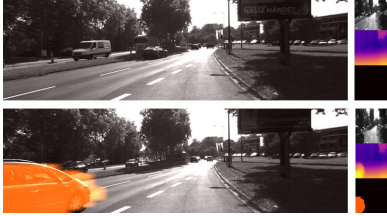
Figure 3. Simple traffic monitoring application. At the right-most position of each frame, we show, from top to bottom, the input 32 \times 32 input image, the depth map inferred by our network from it, and the output of a simple detection system working in the depth domain.
