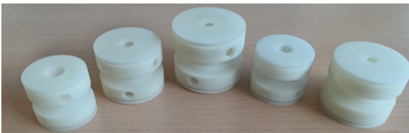
Figure 14: Structures B in PEBA.
