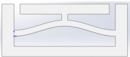
Figure 3: Pre-shaped curved beam.
