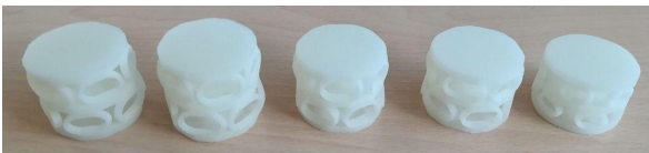
Figure 16: Structures C in PEBA.
