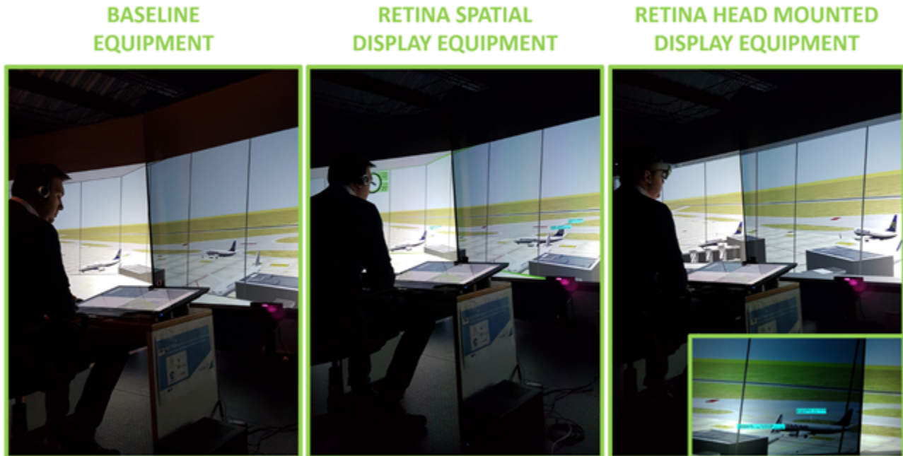
Fig. 2 The baseline equipment (left), the Spatial Display (SD) equipment (center), and the Head Mounted Display (HMD) equipment (right) share the replica of the out-of-the-tower view and a head-down equipment. In addition to that, in the SD equipment (center) overlays are superimposed onto the out-of-the-tower view if the associated object falls within the spatial range of augmentation, i.e. 9 out of 32 tower windows. The HMD equipment (right) shows the same overlays as the SD for each item that falls into the HMD field of view. The HMD operator's personal view is shown at the bottom right corner
