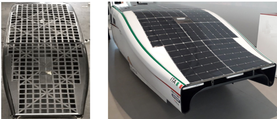
Fig. 12. Final stages of construction of the solar roof: a) the composite sandwich structure is positioned on the vehicle frame; b) the roof is completed with solar panels.
