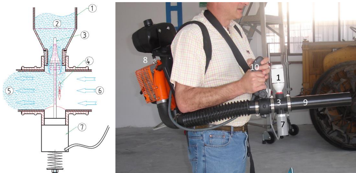
Figure 1. Mechanical blower: 1) bottle containing beneficial organisms - in this case O. laevigatus nymphs; 2) mixture of beneficial organisms and carrier material i.e. buckwheat husk; 3) extraction system; 4) push rod; 5) air stream blowing beneficial arthropods and carrier material; 6) air flow generated by the fan; 7) electromagnet for rod frequency regulation; 8) backpack blower; 9) air diffuser; 10) command lever.
