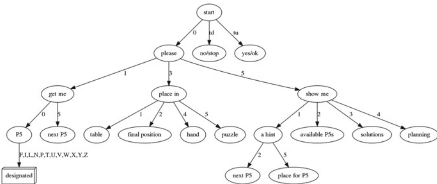
Fig. 7.11 Interaction graph that defines the communication with the robotic agent. Each leaf in the interaction graph correspond to an action performed by the robotic agent
