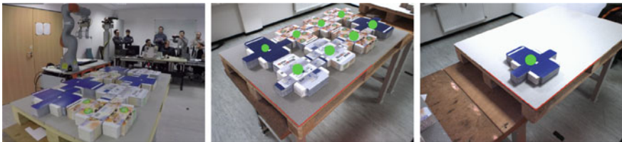
Fig. 7.12 Two pallets and blank piles and their detection results. The red lines in center and right images indicate the pose of pallets, while the green circles indicate the positions of blank piles
