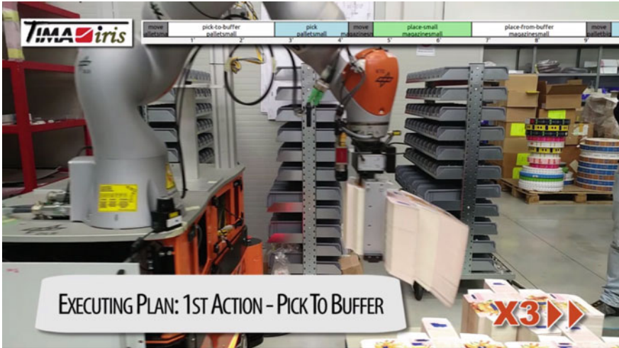
Fig. 7.18 Snapshot of the the robot following the first step of the execution plan
