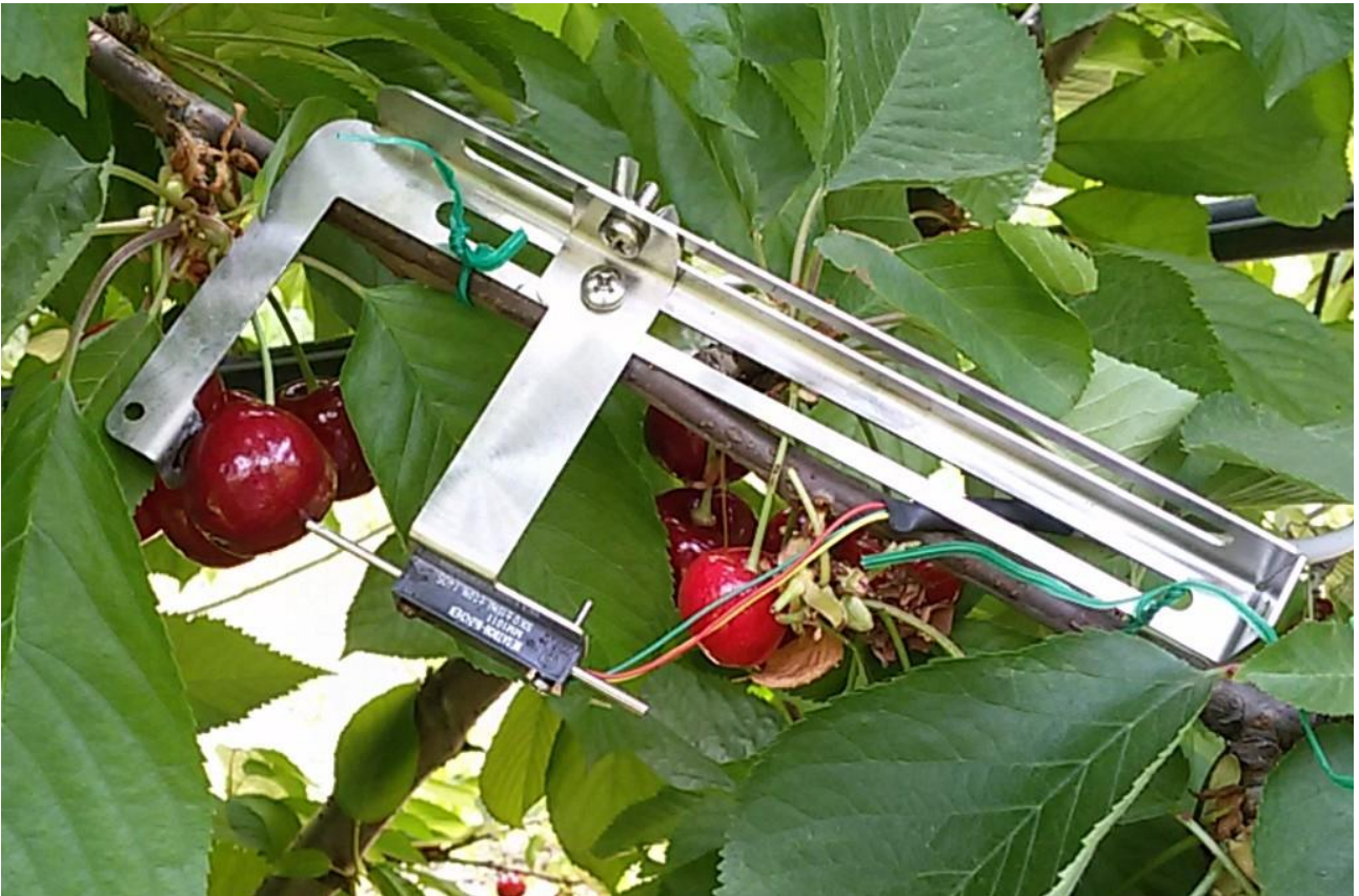
550 551 FIGURE 1 Gauge for the continuous monitoring of fruit growth of ‘Black Star’ sweet cherry at 55 552 DAFB. 553
