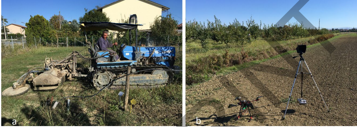
Figure 2. a) Grass mulcher that operates inter row; b) Custom built drone equipped with MApiR Survey 3N NDVI camera
