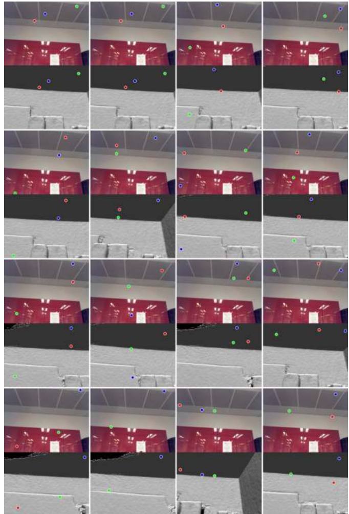
Fig. 20: The top 16 pose candidates (left-to-right, top-to-bottom) corresponding to the failure case from the Pumpkin scene shown in Figure 19. The coloured points indicate the 2D-to-3D correspondences that are used to generate the initial pose hypotheses. Note that in this case, none of the candidates would relocalise the camera successfully, although several are close to being acceptable.
