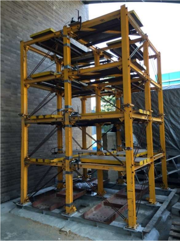
Figure 11. Steel frame structure used for the experimental validation (EERF laboratory, UBC) [13].
