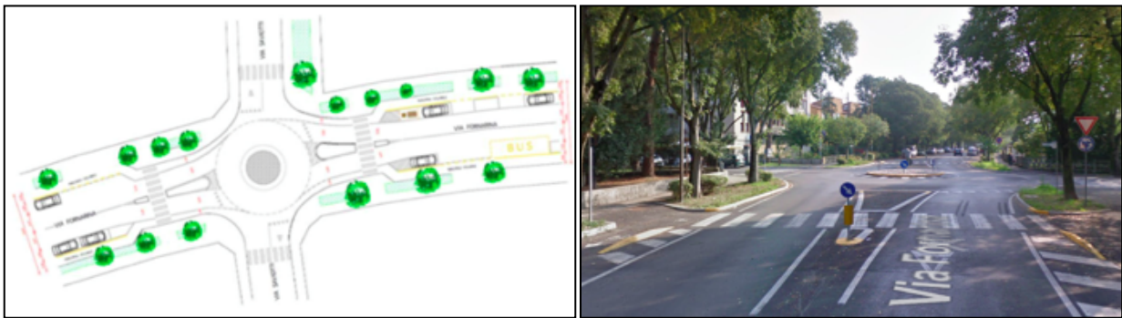
Figure 3. Pedestrian crossing design after the works.
