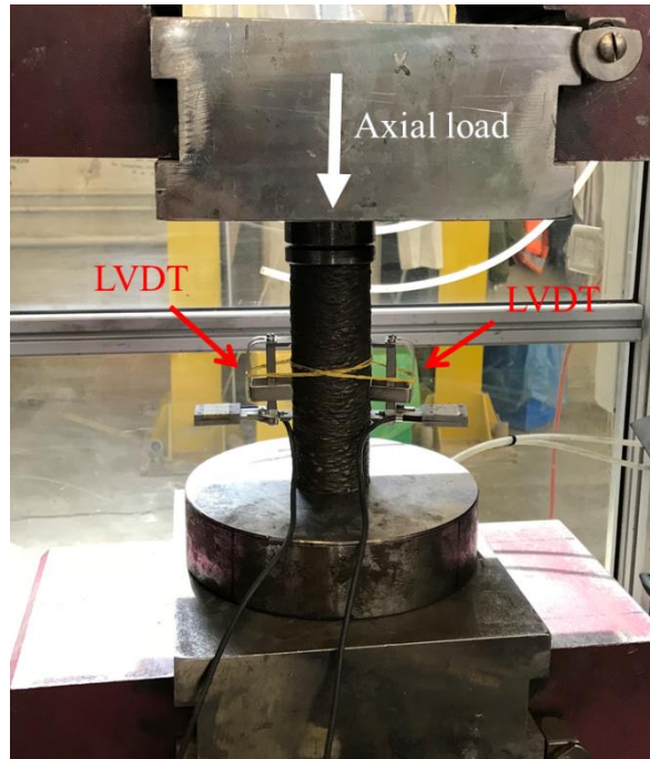
Figure 19: Experimental set-up of the compression tests on stub column specimens.
