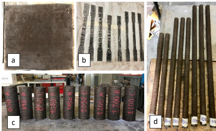
7 8 Figure 6: Specimens produced by MX3D: (a) rectangular plate; (b) “dog-bone” shaped coupons; (c) stub columns. (d) hollow 9 circular tubes.
