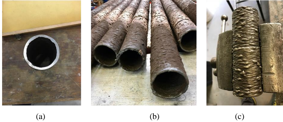
Figure 2: Geometric issues of WAAM tubular elements: (a) irregular cross-section; (b) lack of straightness; (c) surface roughness.
