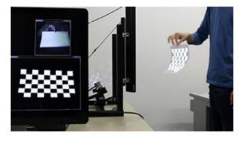
**Fig. 7**: Dynamic projection mapping onto deforming nonrigid surface using a high-speed projector by Gaku Narita, Yoshihiro Watanabe, and Masatoshi Ishikaw from Ishikawa Watanabe Laboratory, Tokyo (2015)
