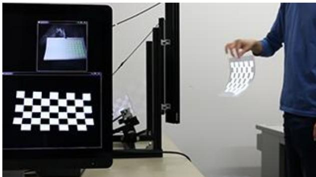
**Fig. 7:** Dynamic projection mapping onto deforming non-rigid surface using a high-speed projector by Gaku Narita, Yoshihiro Watanabe, and Masatoshi Ishikaw from Ishikawa Watanabe Laboratory, Tokyo (2015)
