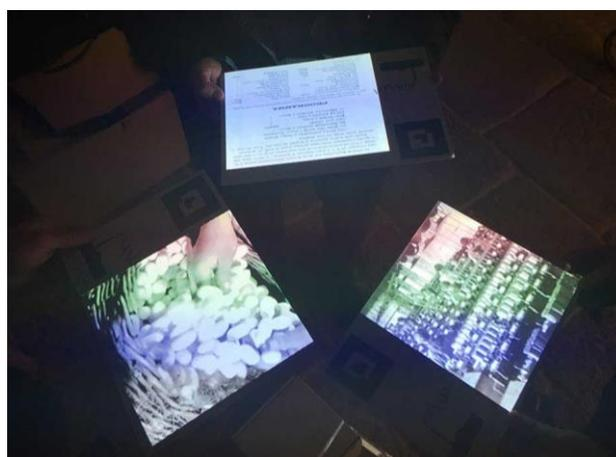
**Fig. 9:** The cardboard panels and the fiducial markers.
