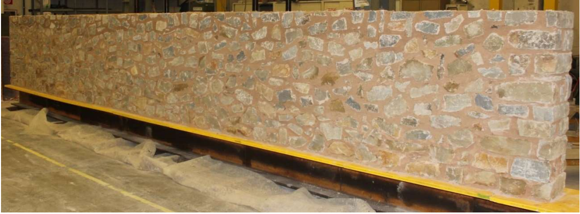
Figure 1. Stone masonry wall.
