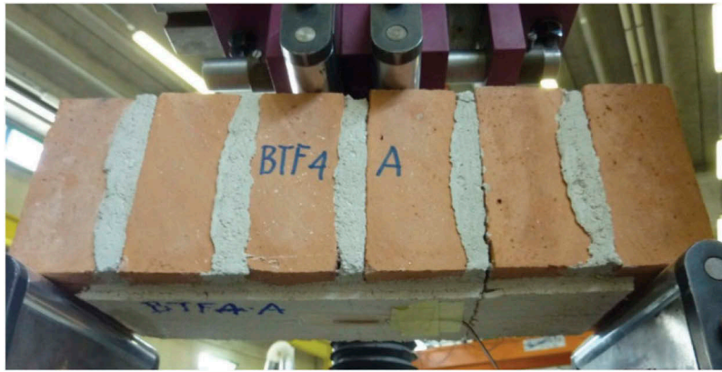
Figure 2. View of the loading set-up for the flexural test of the reinforced masonry stacks.
