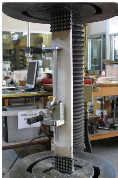
Figure 1. View of the testing set-up for the reinforced mortar plates.
