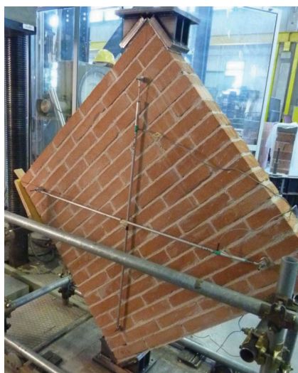
Figure 3. View of the diagonal test set-up.
