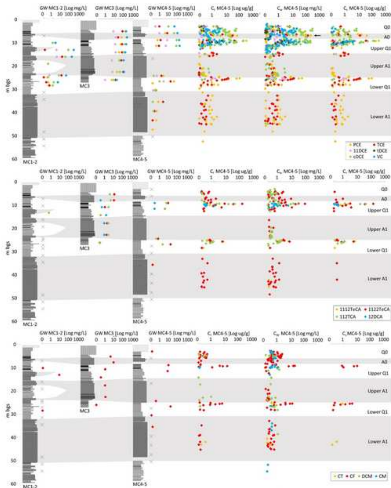
Figure 4: Vertical distribution of chloroethenes (a), chloroethanes (b) and chloromethanes (c). From left: concentrations from groundwater samples (GW; Log mg/L - only concentrations > 0.1 mg/L are plotted for graphical reasons (black crosses indicate GW samples with concentration < 0.1 mg/L for all the analyzed compounds); total concentrations in sediment samples along profile MC4-5 (Ct, Log ug/g - only concentrations > 0.1 ug/g are plotted for graphical reasons); estimated pore water concentrations from phase partitioning (Cw; Log mg/L - only concentrations > 0.1 mg/L are plotted for graphical reasons); estimated sorbed mass concentrations from phase partitioning (Cs; Log ug/g - only concentrations > 0.1 ug/g are plotted for graphical reasons). The one sample with estimated pore water concentration of PCE most likely higher than effective solubility is highlighted with a black arrow. The concentration database is in Tables S2 and S3 of the SM.
