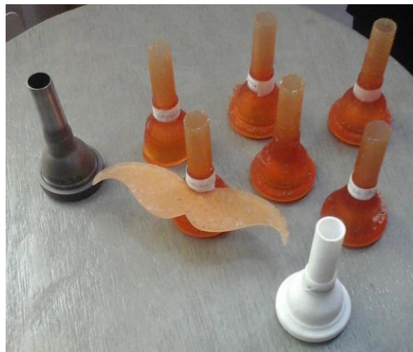
Figure 3 - Original (brass) and manufactured mouthpieces in AM: the orange ones in SLA while the white ones by FDM technology
