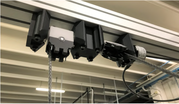
Figure 5. Prototype swivel pulleys.
