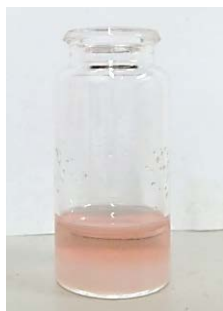
Figure 9: solubility test for URCAT in bidistilled water.
