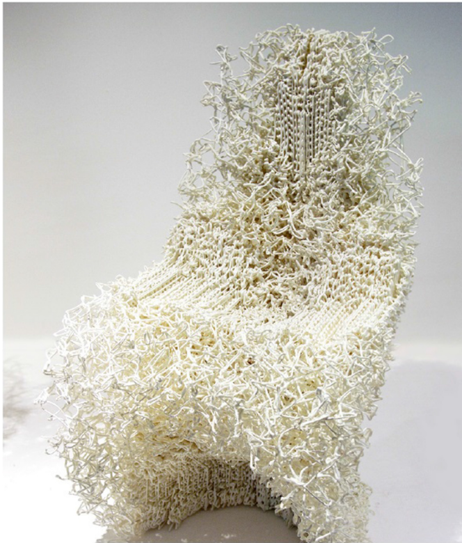
Fig. 13. Pantone chair produced using robotic plastic deposition system [19].
