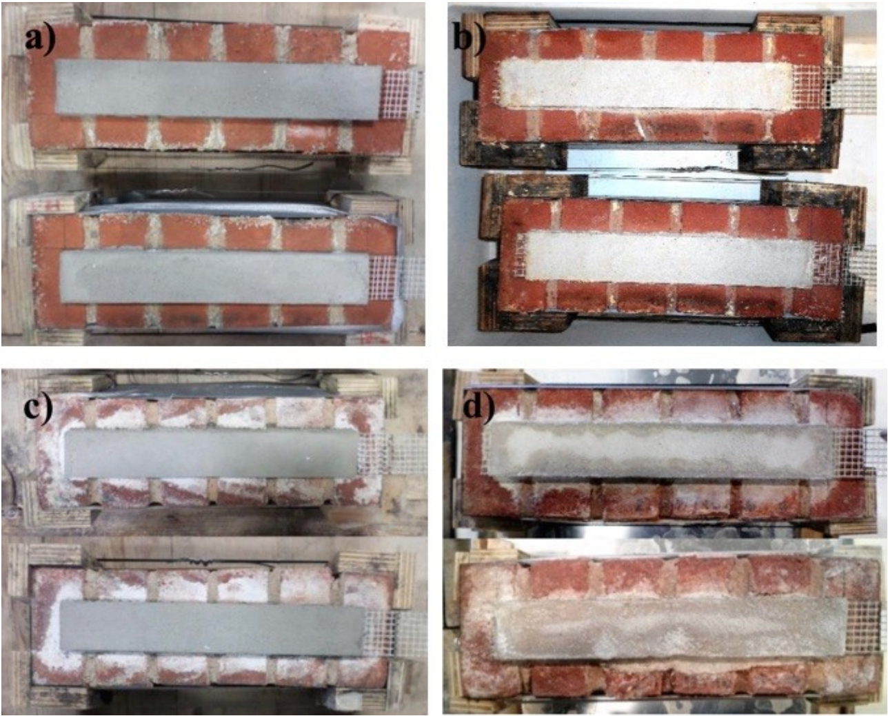
Figure 2. Photos of representative: a) CEM-WAT, b) NHL-WAT, c) CEM-SALT and d) NHL-SALT specimens at the end of the 6 th cycle.
