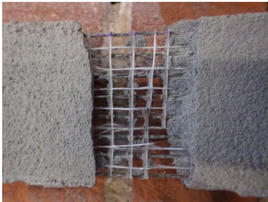
Figure 9. Details of the steel fibers in the composite after the shear test in a CEM-SALT specimens where no surface alterations and/or corrosion are visible.
