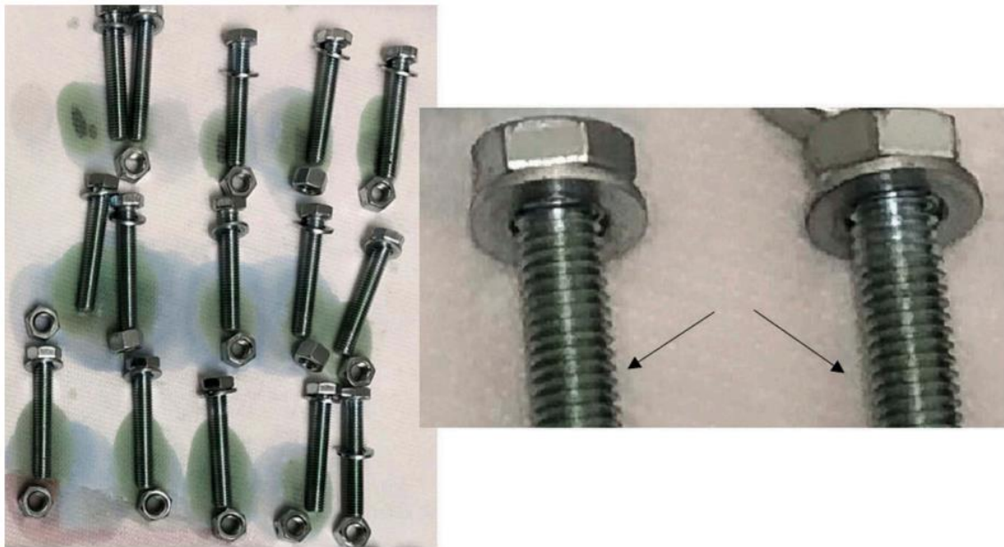
Fig. 10: Screws treated by LOCTITE 270 after untightening: the deposited threadlocker (green color) is well visible in all the threads and highlighted by the arrows in the magnified view.
