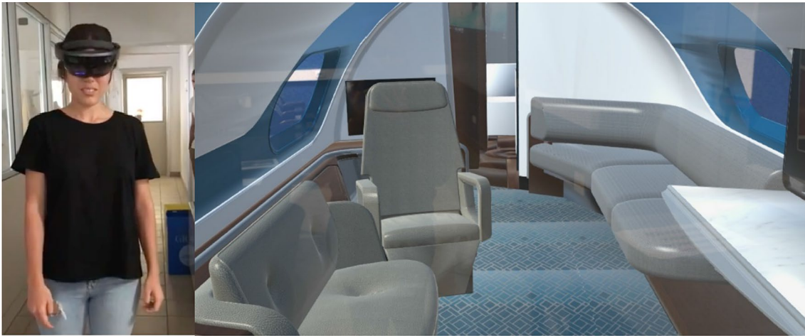
Fig. 6 See-through HMD for subjective visual assessment
