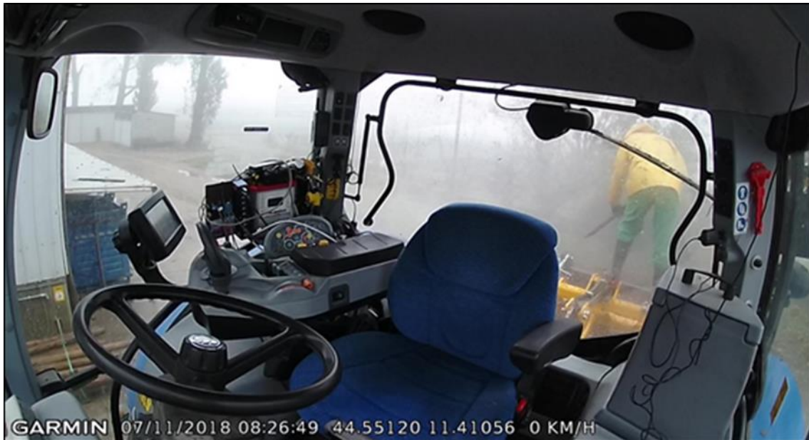
Fig. 8: Frame of a video recorded with the dash cam where the idling stop was caused by washing the tractor.
