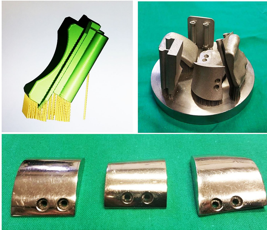
Figure 4. Once the models for the implant sets are sent for manufacturing, these are analyzed first in relevant software for optimal SLM fabrication including position parameters which are suitably set (a typical positioning of the talar component on the top left); in this configuration rough components are manufactured and a platform with a number of these components is produced (top right); these are then extracted and polished with a mirror finishing (bottom).
