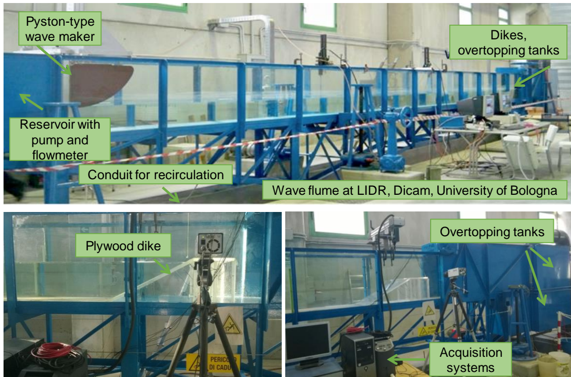
Figure 3 – Wave flume and equipment at the Laboratory of Hydraulics (LIDR), DICAM, University of Bologna.
