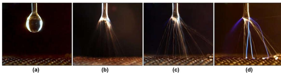
**Figure 2.** Photographs of the electro spraying of water in an 8-mm gap, water flow rate  $0.5 \text{ mL min}^{-1}$ : (a) droplet without a high voltage, (b) electro spray with a high voltage applied, 5.5 kV, (c) electro spray combined with streamer corona, 6.5 kV, (d) electro spray with transition streamer corona-transient spark, 7.8 kV. Reproduced from Machala et al. [55]. All rights reserved.
