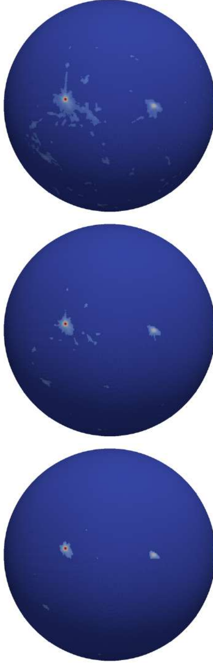
Figure 15: V values after the segmentation as given by Equation 6 for \beta = 0.75 (top), \beta = 0.95 (middle), and \beta = 1.11 (bottom).
