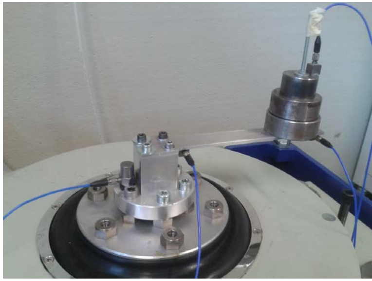
Fig. 6. Experimental setup: the cantilever specimen mounted on the shaker.
