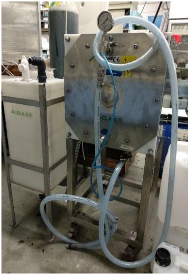
Fig. S1. Picture and flow sheet of the OMW microfiltration plant. The technique implemented in this filtration unit is cross flow filtration, also known as tangential flow filtration, in which the feed suspension passes tangentially along the surface of the filter. A pressure difference drives through the filter the components that are smaller than the pores (average pore-size = 0.2 \mu\text{m} ). The filter contains a network of grooves, all connected to the same outlet line. Components larger than the filter pores are retained and pass along the membrane surface, flowing back to the feed reservoir. The filtration process continues until the pressure required to filter the wastewater exceeds the operational pressure pump threshold, or when the feed wastewater volume is equal to the dead volume of the system (about 4 L).
