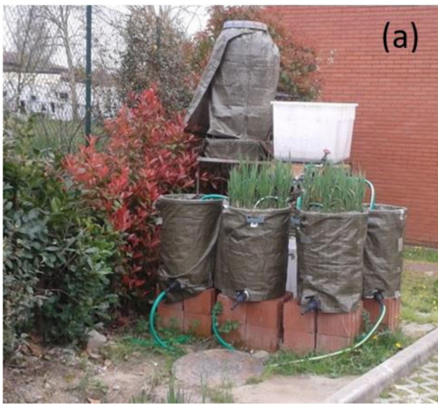
Fig. 1 Pilot plant in March 2016 (a) and a schematic representation of the water flow in the system (b). F Filter, CWw constructed wetland with earthworms, CW constructed wetland, Fw Filter with earthworms. All the systems are vertical flow
