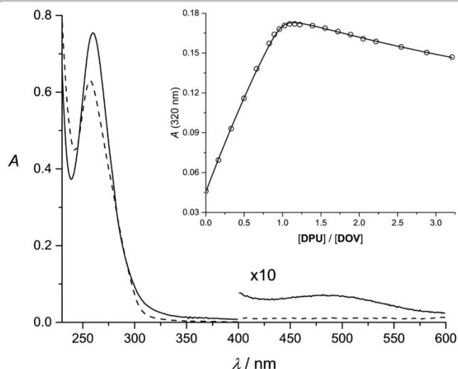
**Figure 9.** Sum of the absorption spectra (dashed line) and the absorption spectrum of the mixture (solid line) of  $\text{CH}_2\text{Cl}_2$  solutions of **DOV** ( $1.4 \times 10^{-5}$  M) and **DPU** ( $1.2 \times 10^{-5}$  M). The inset shows the absorption changes at 320 nm together with the fitted curve upon titration of a  $7.4 \times 10^{-5}$  M solution of **DOV** with concentrated **DPU**.
