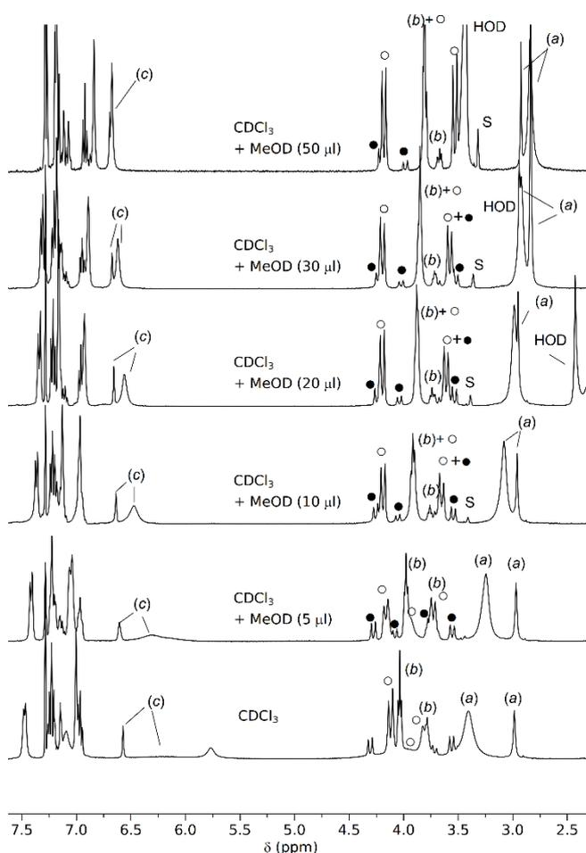
**Figure 5.** NMR stack plot (400 MHz, expanded region, see Fig. S19, SI, for full range) recorded upon addition of increasing amount of  $\text{CD}_3\text{OD}$  to a solution of **DPU** in  $\text{CDCl}_3$  at  $T = 300$  K. The most significant resonances affected by methanol addition have been labelled according to Figure 3.
