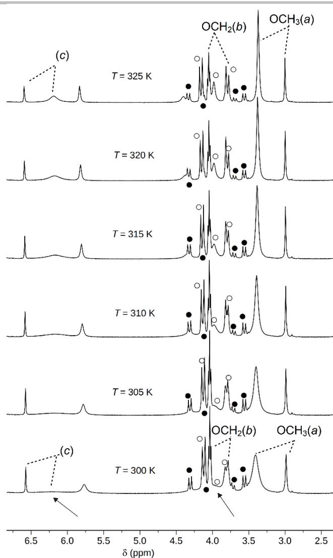
**Figure 3.** Stack plot of the variable temperature NMR experiment ( $T = 300 \rightarrow 325$  K, expanded region, see Fig. S13, SI for the full spectral range) carried out on **DPU** (400 MHz,  $\text{CDCl}_3$ ). The resonances of the bridging methylene protons belonging to conformers **C** and **A-1** (see Figure 2) have been labelled with black and white circles, respectively. Resonances marked as (a), (b) and (c) have been indicated on the molecular sketches of Figure 2.
