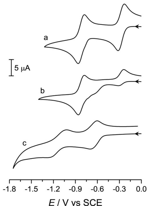
**Figure 11.** Cyclic voltammetric curves for the first and second reduction of the bipyridinium unit in (a) **DOV** ( $c=3.0 \times 10^{-4}$  M), (b) **DPU=DOV** ( $c=3.0 \times 10^{-4}$  M), and (c) **4** ( $c=1.1 \times 10^{-4}$  M) ( $\text{CH}_2\text{Cl}_2$ , 100-fold TBAPF<sub>6</sub>, scan rate 100 mV/s).
