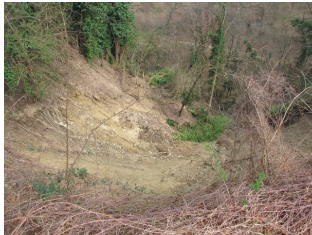
Figure 4. Field photograph of the shallow landslide triggered during the 28 February 2014–2 March 2014 event.
