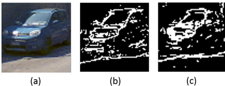
Figure 3: Image of a car taken with a RGB sensor (a) and with our imager (c). Image (b) is obtained by applying the transformation of eq.1-2 on the left RGB image to simulate the in-sensor processing.
