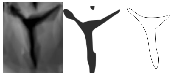
Fig. 11. Vectorization process: (from left to right) a wedge after image processing procedures, binary representation of the wedge, and its vector representation.
