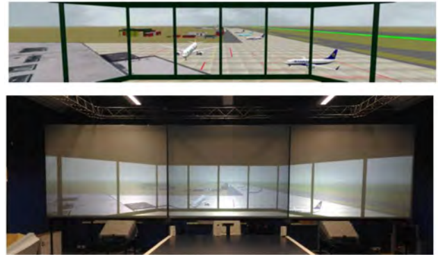
Fig. 7 Out of the Tower view generator: screenshot (top) and deployed and the Reconfigurable Virtual Environment equipped with tracking system (bottom)
