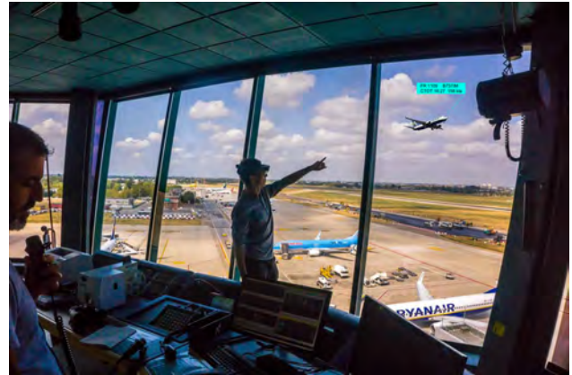
Fig. 1 The RETINA concept is based on the superposition of synthetic overlays onto the real out-of-the-tower view
