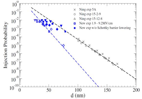
Fig. 2. Injection probability as a function of the distance  $d$  from the Si/SiO<sub>2</sub> interface. Black symbols: Ning experiments [4]. Open blue symbols: experiments carried out on the new devices for different  $E_{ox}$ , reported as functions of  $d$  accounting for barrier lowering. Closed blue symbols: new experiments as functions of  $d$  without barrier lowering. Dashed lines were calculated as  $P_{inj} = A \exp(-d/\lambda)$  following [4].
