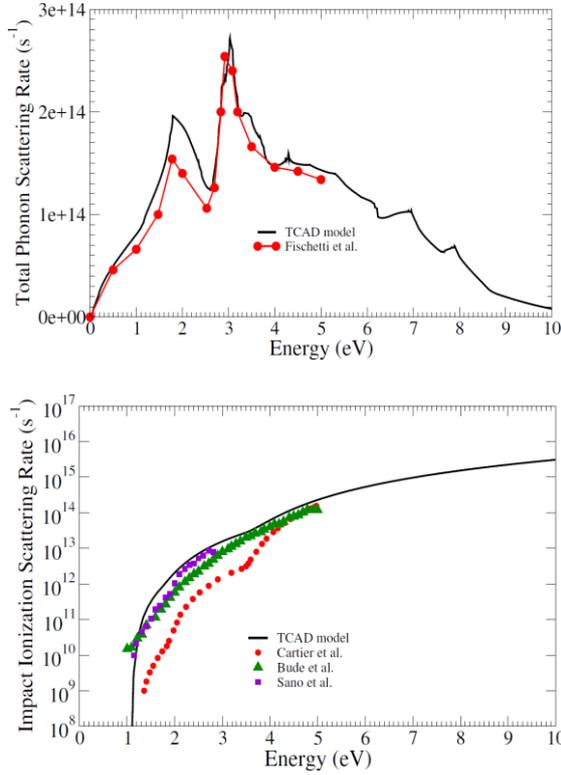
Fig. 3. (Top) Total electron-phonon and (bottom) impact-ionization scattering rates computed with SHE-BTE in comparison with the ones adopted in [5]. Default parameters are used for phonon rate, while a different parameter set is used for the second one.
