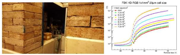
**Figure 5**. (Left) The target region at INFN-LNL used to produce large neutron fluxes for SiPM irradiation: the Be target is visible at the center of the picture. (Right) IV curves for a 20 µm cell SiPM from FBK for various values of the estimated neutron irradiation (neutrons 1 MeV-eq/cm<sup>2</sup>).
