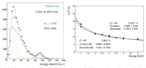
**Figure 3.** Data and Monte Carlo distributions of the total visible energy for a 100 mrad tilt of the calorimeter and a 4 GeV beam of negative pions, muons and electrons in the CERN-PS T9 beamline. (Right): Energy resolution for electrons in data (red point) and Monte Carlo (blue). The fitted parametrization follows the standard form:  $\frac{\sigma(E)}{E} = \frac{\sigma}{\sqrt{E}} + c$ .
