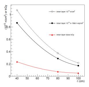
**Figure 1.** (Left): Ionizing dose (red line, kGy), neutron fluence (black dashed line, in n/cm<sup>2</sup>) and 1 MeV equivalent neutron fluence (black continuous line) in the innermost modules of the calorimeter as a function of the tagger radius.
