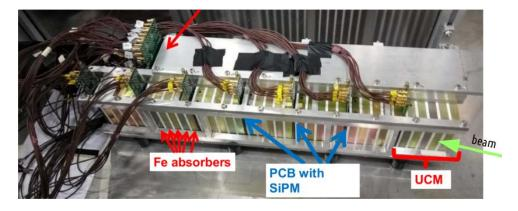
**Figure 2.** The calorimeter exposed at the CERN-PS T9 particle beams. The prototype is composed of an inner part (bottom in the picture) seven calorimetric blocks and a 60 cm long "hadronic" block for the outer part (up in the picture). The compact layout of the light readout is visible through the cabled PCBs.
