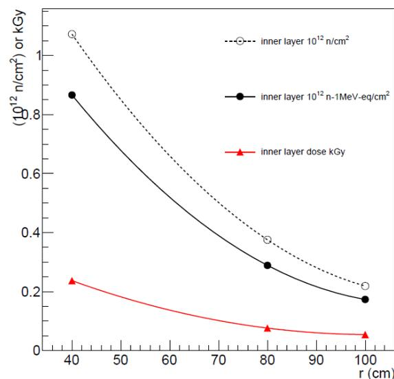
**Figure 1.** (Left): Ionizing dose (red line, kGy), neutron fluence (black dashed line, in n/cm<sup>2</sup>) and 1 MeV equivalent neutron fluence (black continuous line) in the innermost modules of the calorimeter as a function of the tagger radius.
