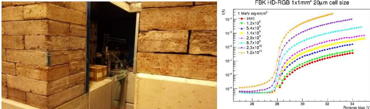
**Figure 5.** (Left) The target region at INFN-LNL used to produce large neutron fluxes for SiPM irradiation: the Be target is visible at the center of the picture. (Right) IV curves for a 20  $\mu\text{m}$  cell SiPM from FBK for various values of the estimated neutron irradiation (neutrons 1 MeV-eq/cm<sup>2</sup>).
