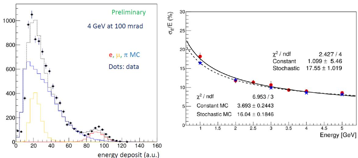
**Figure 3.** Data and Monte Carlo distributions of the total visible energy for a 100 mrad tilt of the calorimeter and a 4 GeV beam of negative pions, muons and electrons in the CERN-PS T9 beamline. (Right): Energy resolution for electrons in data (red point) and Monte Carlo (blue). The fitted parametrization follows the standard form:  $\frac{\sigma(E)}{E} = \frac{\sigma}{\sqrt{E}} + c$ .
