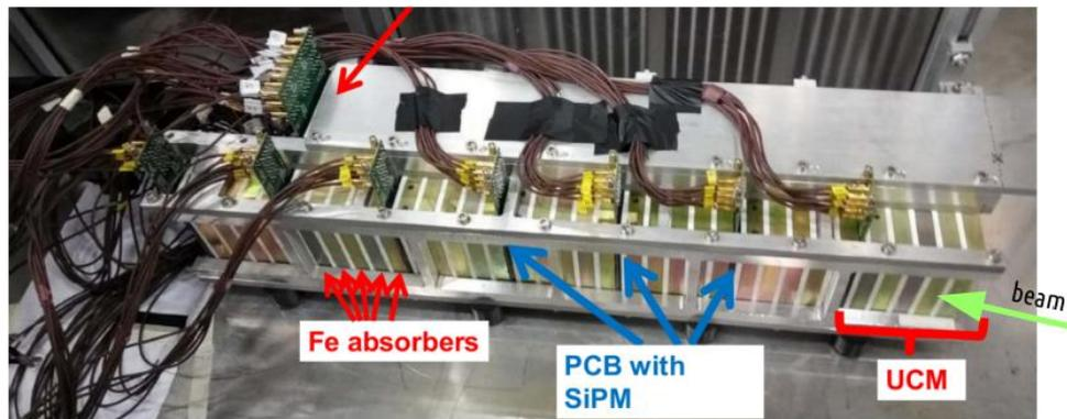
**Figure 2.** The calorimeter exposed at the CERN-PS T9 particle beams. The prototype is composed of an inner part (bottom in the picture) seven calorimetric blocks and a 60 cm long “hadronic” block for the outer part (up in the picture). The compact layout of the light readout is visible through the cabled PCBs.
