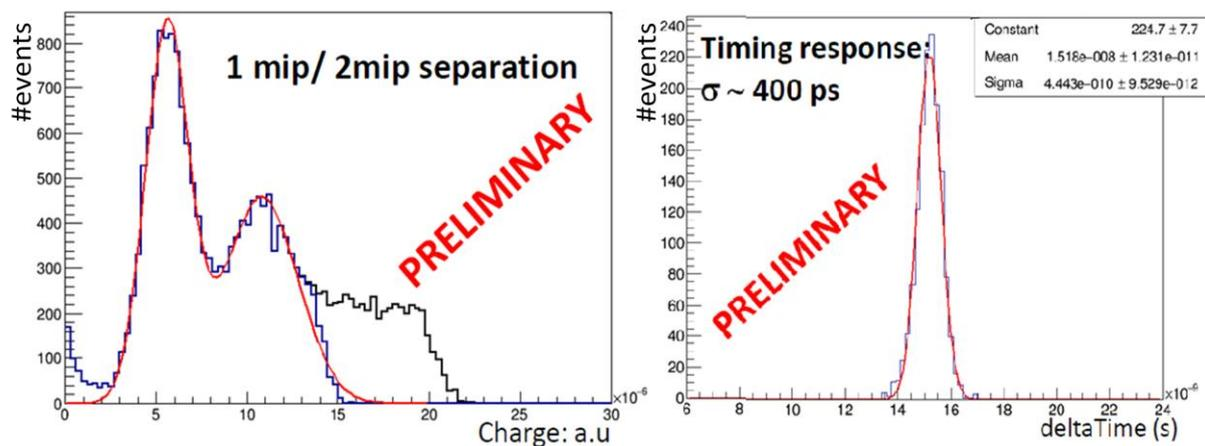
**Figure 4.** (left)  $e^+e^-$  couples produced from the  $\pi^0$  decay: it's visible the separation between 1 particle and 2 particles. (right) timing measurements performed with a fast scintillator used as trigger, the resolution of ~400 ps.
