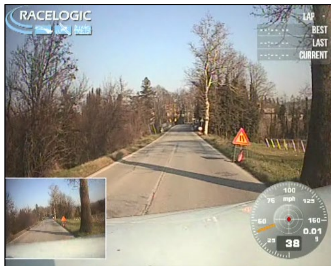
Figure 2: Video V-Box (bottom) and Mobile Eye Tracker (top) synchronization for the computation of the distance of first-fixation to a road sign.
