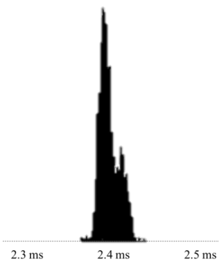
Fig. 5 Pdf of the voltage phase acquired with the oscilloscope
