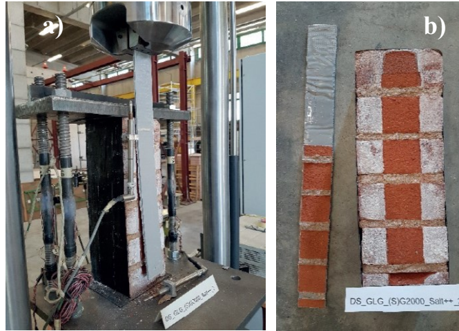
Figure 2. (a) Direct shear test set-up and (b) debonding with cohesive fracture of the support of SRP specimens.
