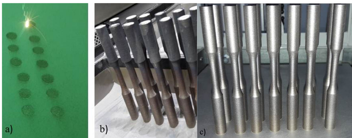
Fig. 3 - (a) As Built specimens during scanning, (b) Specimens cleaning from powder, (c) Specimens after micro-shot-peening
