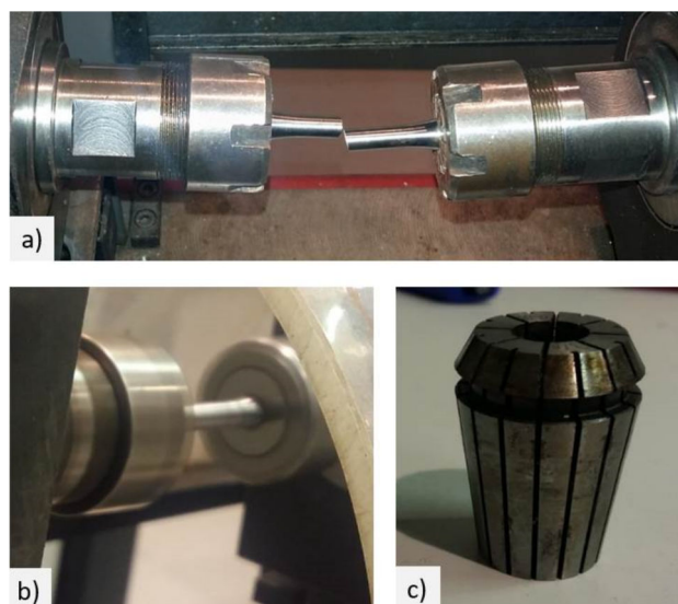
Fig. 4 - (a) Clamped specimen after breakage, (b) Specimen running, (c) Chuck collet
