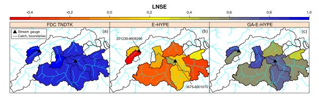
**Figure 10.** Spatial distribution of Nash–Sutcliffe efficiency computed for log-transformed streamflows (LNSEs) at the 11 E-HYPE prediction nodes considered in the study: geostatistically predicted flow–duration curves (FDC TNDTK, **a**); predicted daily streamflow time series (E-HYPE, **b**, and GAE-HYPE, **c**, respectively); the locations of the two sites considered in Figs. 9 and 8 are highlighted with black triangles.
