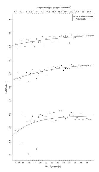
**Figure 11.** LNSE ratio (see Eq. 12) as a function of stream gauge availability: black dots represent the average of 11 LNSE ratio values, while crosses indicate their 95 % confidence interval.
