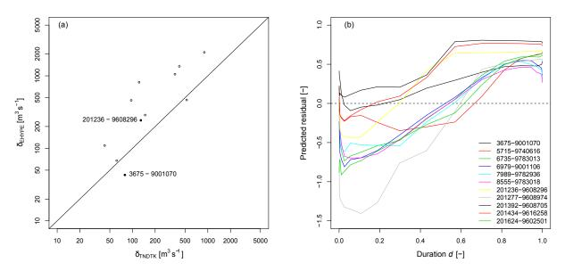
**Figure 7.** 11 E-HYPE prediction nodes: (a) comparison between TNDTK (x axis) and E-HYPE (y axis) in terms of distances  $\delta$ s between empirical and predicted FDCs; the 1:1 line represents equivalent performance for TNDTK and E-HYPE; (b) standardized residual—duration curves computed as illustrated in Eq. (8) (TNDTK streamflow quantiles are used for standardization).
