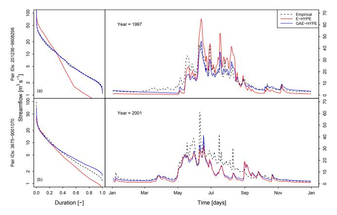
**Figure 8.** Examples of comparison between observed streamflow series (black dashed lines) and simulated daily streamflows via E-HYPE (red solid lines) and GAE-HYPE (blue solid lines) for two representative sites and a given year, showing two cases for which the geostatistical assimilation procedure resulted in sizeable (a) and limited (b) improvements, respectively.
