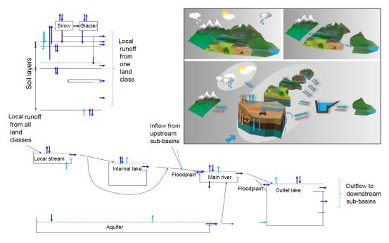
Figure 4. Schematic concept of the HYPE model (all equations are available at http://hypecode.smhi.se/, last access: 30 July 2018).
