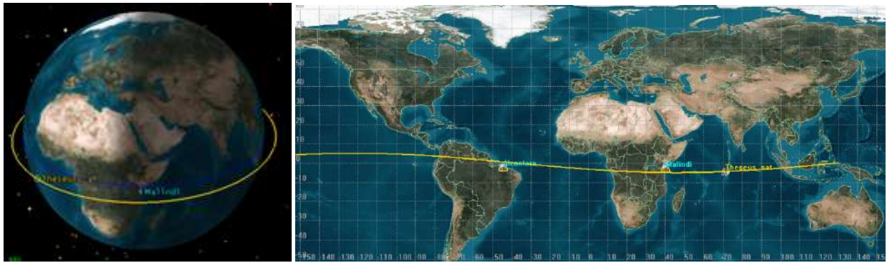
Figure 44: THESEUS Orbit Configuration (Left) and THESEUS Orbit Ground Track (Right).
