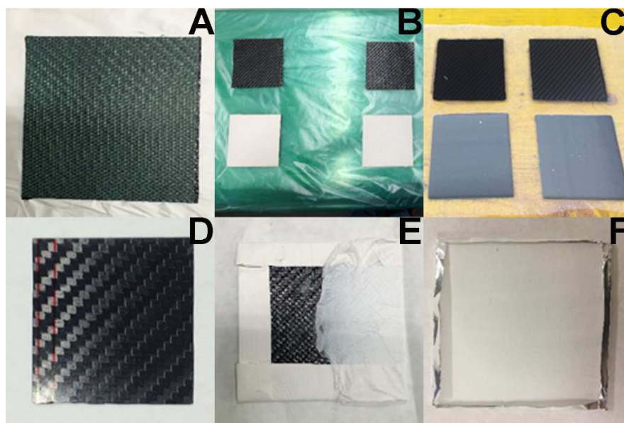
Figure 1. C-Neat sample (A), C-PMIA inc W sample (B and C), CP-Neat sample (D) and CP-PMIA W sample (E and F) at different stages of the covering procedure.
