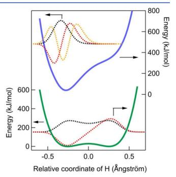
Figure 3.Left and right axes: potential curves of ACAC in the ground state (PES-gs, thick green curve) and core ionized state (PES-ion, thick blue curve). The amplitudes of the vibrational wave functions (in arbitrary units, scale not shown) for the ground states (black curves), the first excited states (red curves), and the second excited state (yellow curve) of the proton in the ground/core ionized states are also shown.
