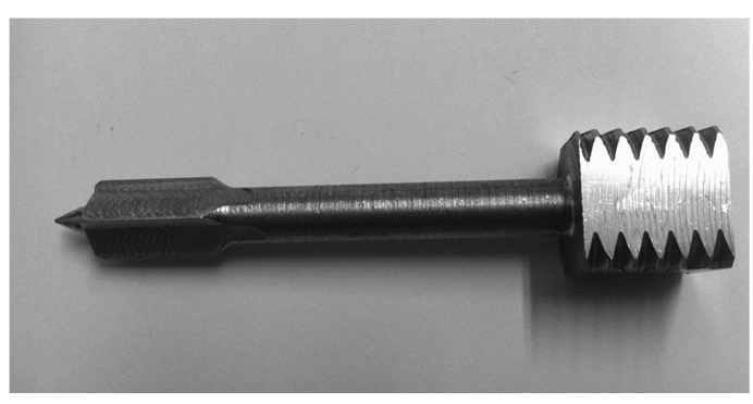
116 Figure 1 - Novel nail proposed for the Torque Penetrometric Test of historical mortars [21].
